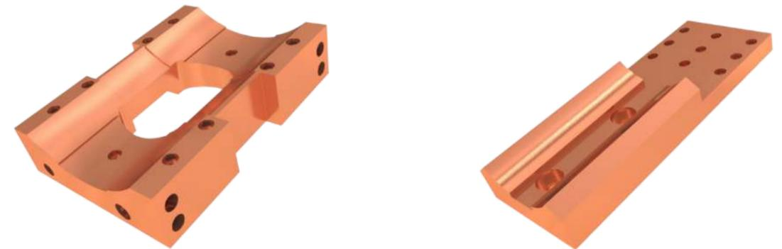
The "Forged" Type is produced by making a specific forge mould or directly by forging a copper block or a semi-prepared moulded part which its dimensions are close to the final one; this model's electrical conductivity is above 101% of IACS and is more consistent. Thus, the forged model is more reliable compared with the Moulded one and of course, final price is higher compared with moulded types.
